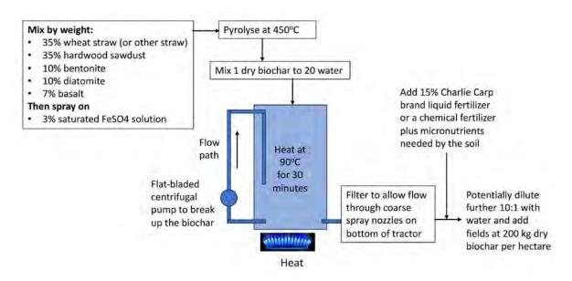
Figure 7.15 A method to make a liquid biochar fertiliser
