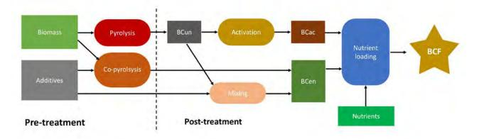
**Figure 7.4** Simplified representation of biochar compound fertiliser (BCF) production processes, where BCun, BCac, and BCen are biochars that are untreated, activated, and enhanced, respectively. Material types are in rectangles and processes in ellipses. (Modified from Rasse et al.<sup>7</sup>)
