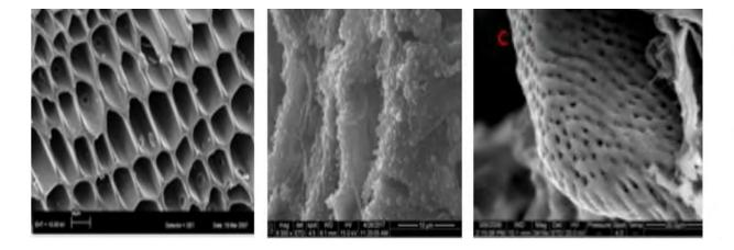
**Figure 4.2** The pore structure of biochars. Left, fresh wood biochar. Middle, the dramatic changes occurring on the surfaces of biochar after 12 months in soil. Right, biochar made at 550°C from chicken litter shows lowered porosity due to melted minerals.
