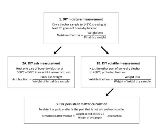
**Figure 11.1** Analytic sequence for determining the prime constituents of biochar using simple do-it-yourself (DIY) methods. Note the formulae express the various fractions on a dry basis (db); i.e. relative to the final dry weight. If multiplied by 100 the fractions become percentage contents (db)
