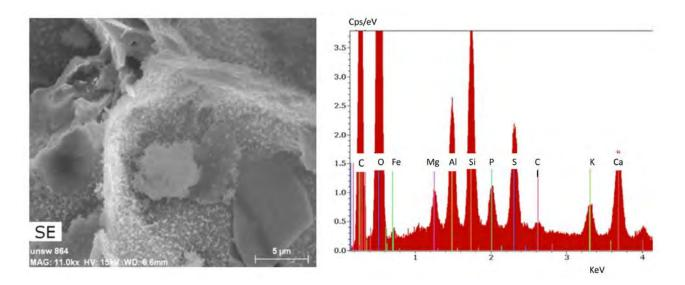
**Figure 7.3** An electron microscope image of a mixed-feedstock biochar pyrolysed from wood and manure at 450°C–600°C in a simple kiln (TLUD). The woody biochar is coated in very fine particles of minerals and nutrients. The spectrum shows high contents of Mg, Ca, P, and S. Very high levels of Al and Si in the spectrum are from the clay that was on the straw collected from the fields. There was no nitrogen, possibly due to the high temperature of production
