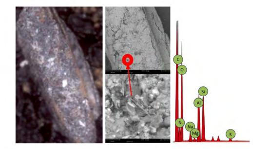
**Figure 8.15 Left:** Rhodes grass seed coated with a mixture of bentonite, diatomite, and biochar. **Middle:** Scanning Electron Microscope image of the coating on the seed showing tiny pieces of biochar bonded with bentonite and diatomite. **Right:** X-ray analysis of biochar indicating that it has high content of N and small amounts of Mg, Na, Cl, S, and K. Modified from Maraseeds<sup>13</sup>
