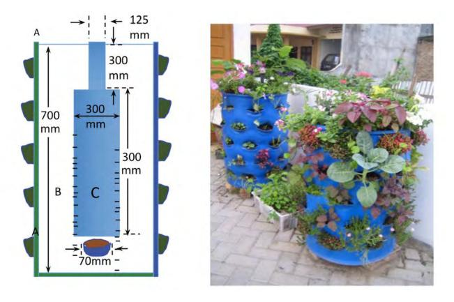
Figure 8.18 Biochar garden for a small space in Indonesia. A, plastic barrel with shaped pockets; B, soil with biochar; C, central buckets with vegetable scraps, worms, and biochar
