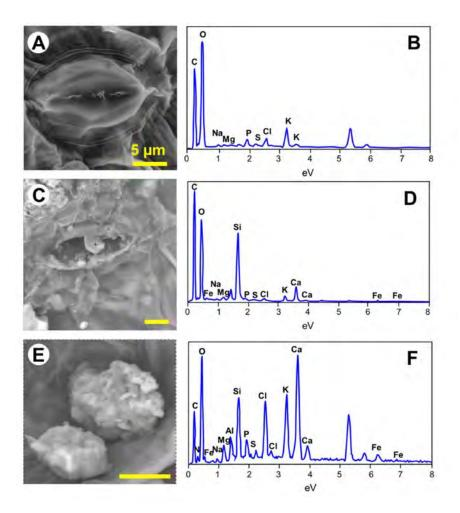
**Figure 6.8** Scanning electron microscopy images and elemental analysis of biochar and carbon-coated minerals inside and around stomata. **Top:** Stomata. **Middle:** Biochar-treated leaf with stomata and organo-mineral complexes. **Bottom:** High-resolution image of organo-minerals inside the stomata<sup>16</sup>
