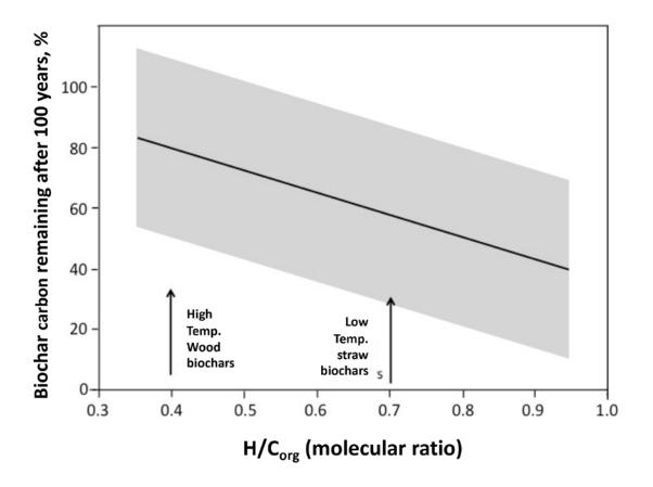
**Figure 4.6** The percentage of the biochar carbon remaining in the soil after 100 years as a function of  $H/C_{organic}$ . The solid line represents the mean correlation of the biochars measured. The grey band represents the prediction interval within which 95% of future biochar measurements are expected to fall. (Modified from Budai et al.<sup>4</sup>)
