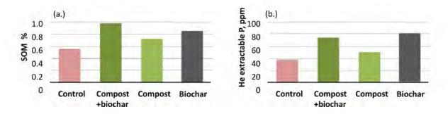
**Figure 8.13** Increase in soil organic matter (SOM) and extractable P following application of biochar, compost, and both to vineyards on sandy soil, King City, California, 2019-2022<sup>12</sup>
