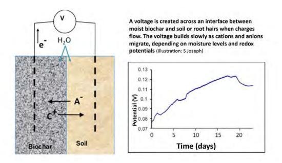
**Figure 4.14** Biochar with water in its pores can store and donate electrons and ions like a battery. In the soil, it creates a potential difference between biochar and the soil, affecting electron activity. C<sup>+</sup> represents the positively charged cations such as potassium and A<sup>-</sup> represents negatively charged anions such as nitrates.
