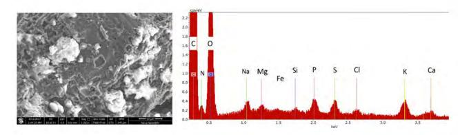
**Figure 5.4** Organo-mineral clusters on a high-temperature wood biochar taken from the gut of a worm. Note the relatively high nitrogen (N), potassium (K) and phosphorus (P) contents in the X-ray spectrum
