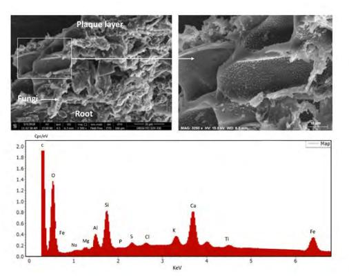
**Figure 6.4 Top Left:** A piece of wheat straw biochar embedded in the soil layer that forms on rice roots. **Top Right:** A magnified image of the embedded biochar particle. Fine mineral-nanoparticles coat the biochar pore surfaces. **Bottom:** X-ray analysis of the magnified area showing high contents of some nutrients on the surface of the biochar. The nutrients can be available for uptake by the plant
