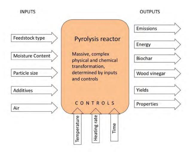
Figure 1.7 Dynamics of the pyrolysis process
