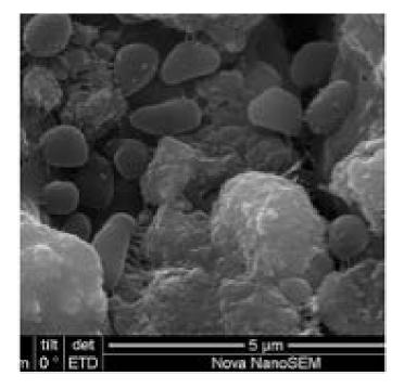
**Figure 7.11** Scanning electron microscope image of microbes growing on the post-treated biochar that is depicted in Figure 7.10
