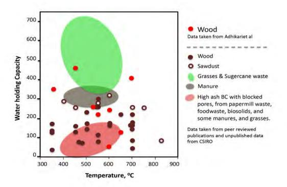
**Figure 4.4** Water-Holding Capacities of over 60 biochars (BC) as a function of temperature. Individual data points are shown for wood and sawdust BCs produced between 350 and 830°C. Similar data points for biochars produced between 400 and 600°C from grasses, manures, and high ash feedstocks are indicated by their approximate ranges of WHC. (Data from an unpublished CSIRO study.)
