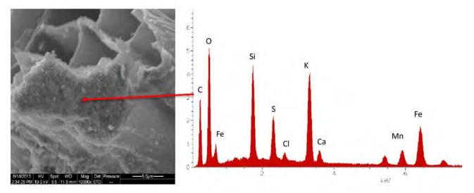
**Figure 5.3** High-temperature wood biochar after composting, showing formation of organo-mineral clusters on the surface of a macropore. The X-Ray dispersive analysis shows high concentrations of K (potassium), S (sulphur), Si (Silica), Fe (iron) and small concentrations of Mn, Cl, and Ca
