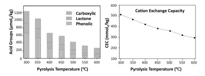
**Figure 4.11** Acidic functional groups (phenolic, lactone, and carboxylic) and cation exchange capacity (CEC) of poultry litter biochars generated at different pyrolysis temperatures. (Redrawn from Song & Guo 2011.<sup>12</sup>)
