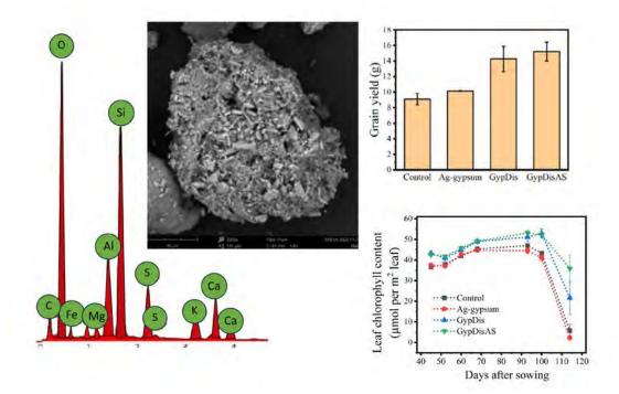
**Figure 7.7 Left:** Scanning electron microscope image and elemental analysis of a biochar–gypsum particle. **Top right:** the yield of wheat per pot for Control = no amendment, Ag-gypsum = Agricultural gypsum at 500 kg/ha, GypDis = liquid-gypsum-coated biochar, and GypDisAS = liquid-gypsum biochar with Aquasil dispersant. Bottom **right:** leaf chlorophyll content resulting from the four treatments. (Information provided by Dr E Tavakkoli)
