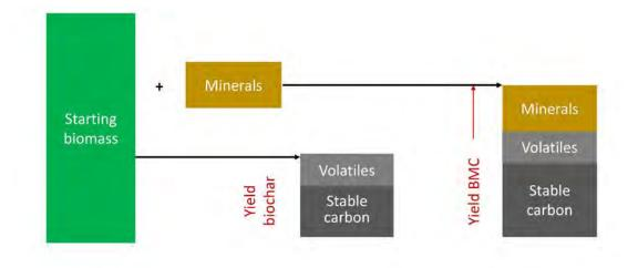
**Figure 7.5** Effect of mixing minerals with biomass on yield of stable carbon after pyrolysis. Minerals increase the yield of both biochar and the stable carbon fraction of the biochar. The minerals "complex" with the biochar to form a greater yield of biochar-mineral-complex (BMC)<sup>14</sup>
