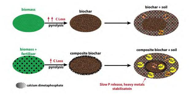
**Figure 7.6** Schematic of adding a high-P mineral or chemical to biomass and co-pyrolysing to improve biochar carbon retention, slow nutrient release, and stabilise heavy metals in soils.<sup>17</sup>
