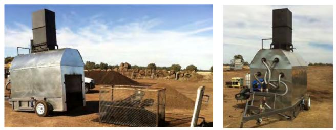
**Figure 3.6** The Big Roo 4 cum portable batch kiln designed for straw. (<u>www.allthingsbiochar.com.au</u> for further information)
