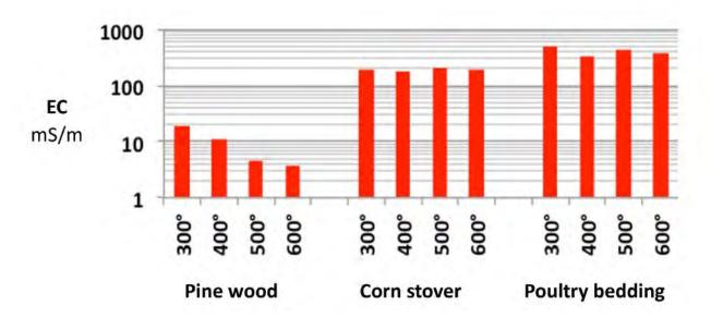
**Figure 4.9** EC for three different biochars, plotted on a log scale, as a function of temperature. The ECs of biochars from corn stover (stalks) are 10 to 50 times higher than those of the wood biochars, while the ECs of manure biochars are 1.5 to 2.5 times higher than those of the corn stover. (Data from Rajkovich.<sup>7</sup>)
