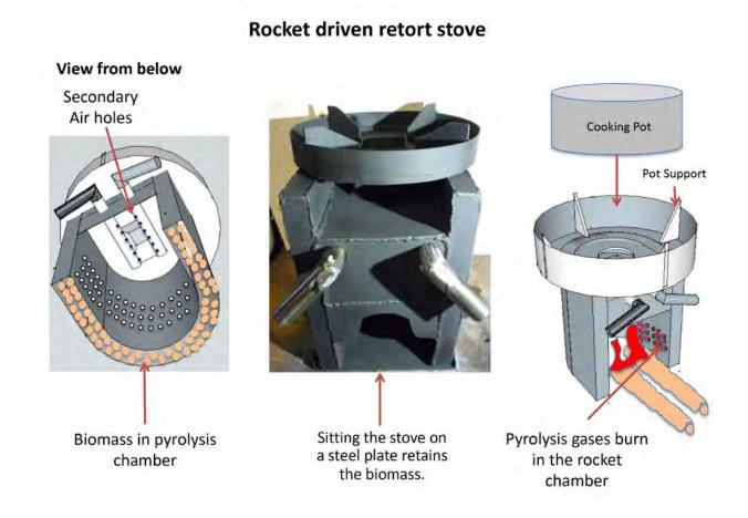
Figure 3.4 A rocket driven retort stove used for rice husk pyrolysis. (Photo Stephen Joseph)
