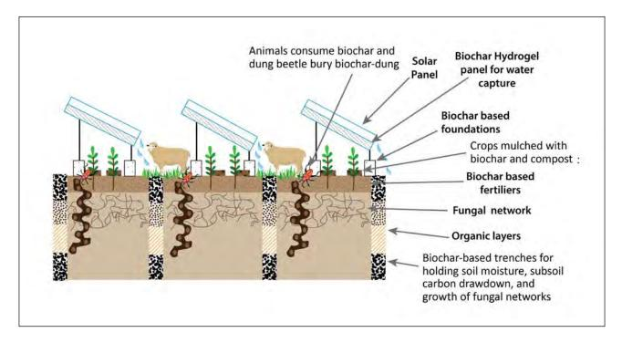
Figure 10.6 Integrating biochar underneath and between solar arrays (S. Joseph)
