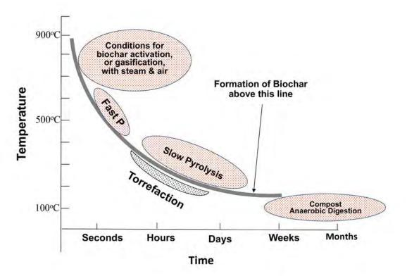
**Figure 1.6** A schematic of the effect of time and temperature on formation of biochar and the operating zones for different thermal and microbial processes. Temperature and time ranges are approximate and schematic.
