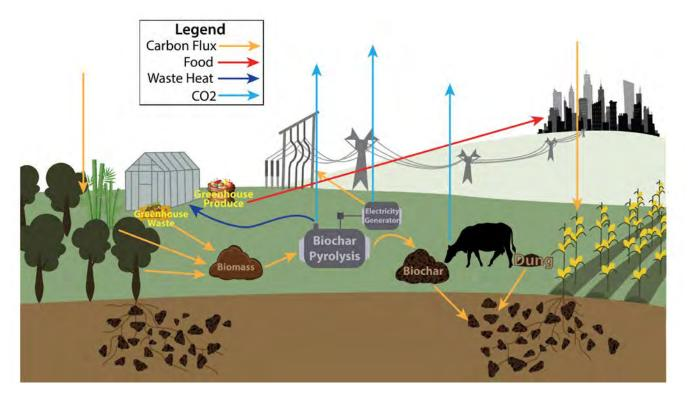
Figure 10.5 Potential energy utilisation pathways and carbon fluxes for heat, electricity, and biochar generated during biomass pyrolysis.<sup>8</sup>
