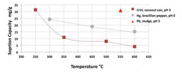
**Figure 4.13** Capacity of selected biochars produced at different temperatures for metal sorption from aqueous solutions. The legend lists in order: Heavy metal species, feedstock, biochar pH. (Data from Li et al. 2017.<sup>14</sup>)
