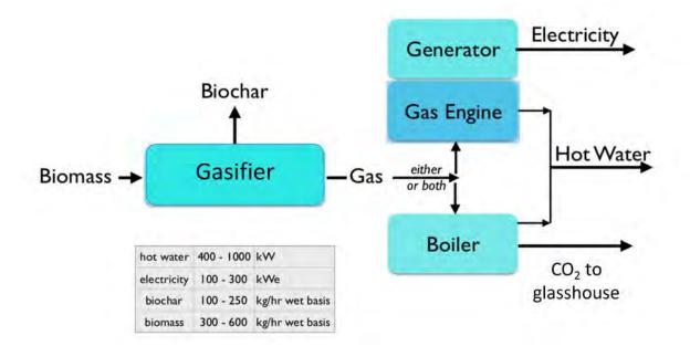
**Figure 3.12** Rainbow Bee Eater ECHO2 biomass to energy system for producing heat and electricity and, optionally, clean CO<sub>2</sub> rich boiler exhaust for greenhouse heating. <u>www.rainbowbeeeater.com.au</u>
