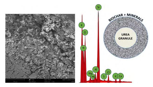
**Figure 7.13** Biochar-plus-mineral encapsulated urea. **Left:** Scanning electron microscope image of the biochar–mineral surface. Centre: Elemental analysis shows the high nitrogen content that has infused into the surface. **Right:** Schematic depiction
