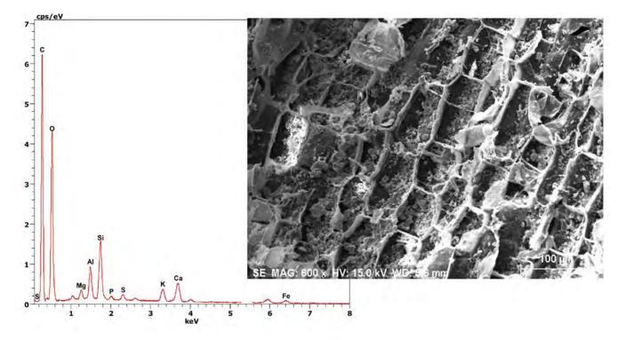
**Figure 2.3** Scanning electron microscope examination of biochar from a millet field showing the carbon matrix filled with minerals available for plant and microbes. The four largest peaks in the X-ray spectrum are C, O, Si, and Al.<sup>3</sup>
