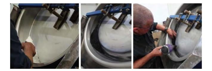
**Figure 7.14** Coating urea granules. **Left:** Adding a mixture of damp clay and biochar powder to urea granules in a plate agglomerator. Middle: The clay and biochar are coating the urea granules. **Right:** Drying the granules with a hair dryer
