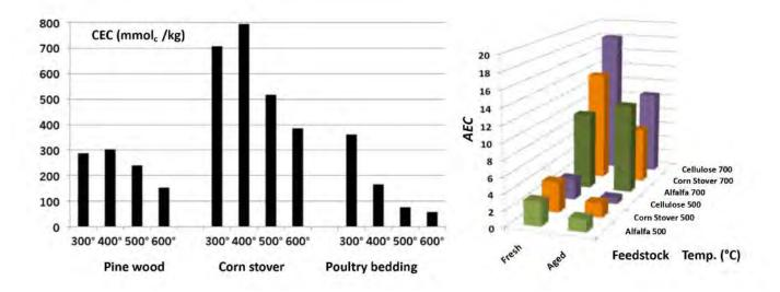
**Figure 4.12** Left: Available CEC for biochars at different feedstocks and temperatures (adapted from Rajkovich<sup>7</sup>). Right: Anion exchange capacity of fresh and 4-month aged biochars from different feedstocks and biochar production temperatures. (Adapted from Lawrinenko.<sup>13</sup>)
