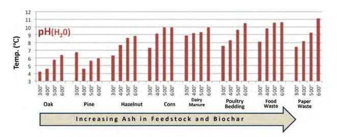
Figure 4.8 pH of a range of biochars produced at different temperatures (data from Rajkovich<sup>7</sup>).
