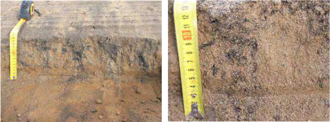
Figure 6. Rotary hoe incorporated wheat (left image) and mallee (left image) biochar at rates of 60 t/ha in the soil at Kalannie, showing depth of placement and degree of incorporation.
