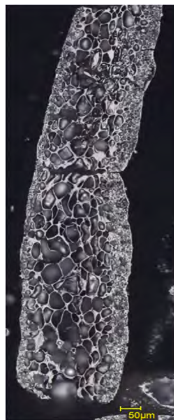
Fig. 9. A typical example of an inertinite maceral in biochar, captured in a white-light photomicrograph.
